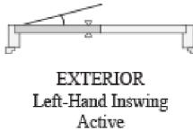
Left Hand Inswing, Stainless Steel Ball Bearing Hinges,
